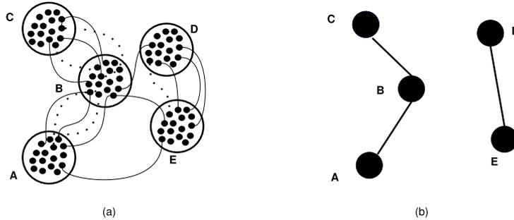
**Fig. 1.** Example of reduced graph creation. Left: original regular partition. Here, only the pairs  $(A, B)$ ,  $(B, C)$  and  $(D, E)$  are regular. Right: the graph obtained after the reduction process.
